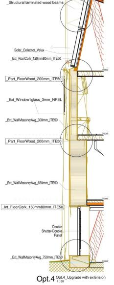
Section of Opt.4 proposal: 450€/sqm provide for a new seismic structure and 10 sqm extension, the local maximum expansion limit.
