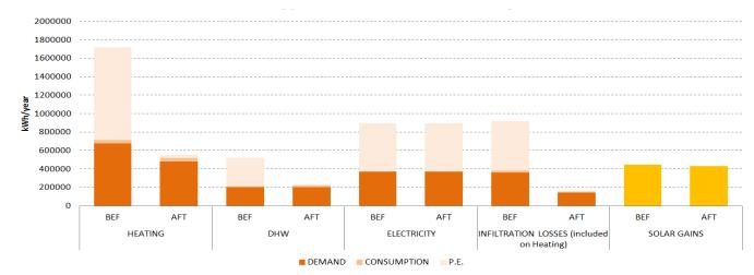
Building energy performance (Conversion Factors: Electricity 2,.4; Natural Gas: 1,.07; Source: IDAE // Infiltration before renovation: 0,6
