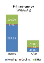
Figure above on the left shows the energy needs for heating, cooling and DHW before and after the renovation works calculated in accordance with the Portuguese thermal codes, which consider the comfort indoor temperatures of 20°C in winter and 25°C in summer.
