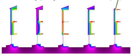
Thermal behavior analysis of the intervention options above using THERM (LBNL, 2015). Notice that Opt.1 denotes severe thermal stress in the floor area and lower temperatures inside the walls that may result in frost damage in colder nights.
