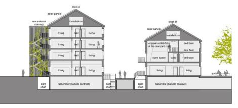
Cross section of block A (to the left) and block B (to the right) after the renovation.
